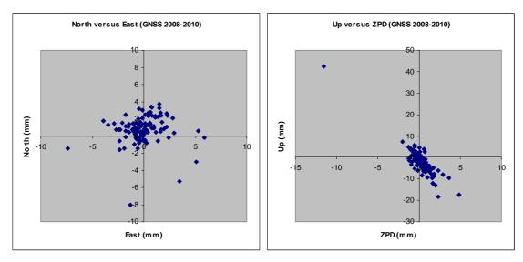
Fig. 7: GLONASS-GPS translation parameter results concerning N/E and U/ZPD, plotted for "GNSS-only" test analysis covering 3 years (2008–2010).
