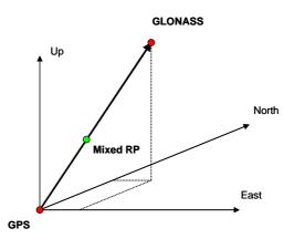
Fig. 1: GLONASS-GPS intersystem translation parameters with respect to station coordinates.
