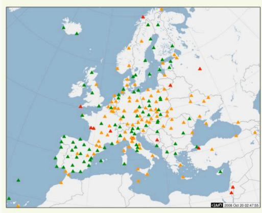
The GNSS data from the EPN stations are freely available through the internet. Depending on the station data policy, daily (mandatory), hourly RINEX (92.2% of the EPN stations) 15min high-rate RINEX (from real-time streams) and real-time (42.2% of the EPN stations) data are made available (see map).
