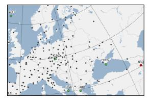
Fig. 1 : EUREF permanent GNSS tracking network (status June 2011); green dots: the stations added to the network since June 2010; red dots: station that was withdrawn from the EPN.
