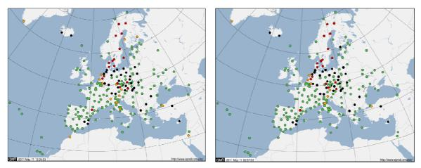
Fig. 4: Overview of the absolute receiver antenna calibrations used in the EPN analysis. Left: using epn\_05.atx, right using epn\_08.atx. Black: individual calibrations, green: robot calibrations, orange: from field/relative calibrations, red: uncalibrated radome. The circles indicate regions were a clear improvement is seen.
