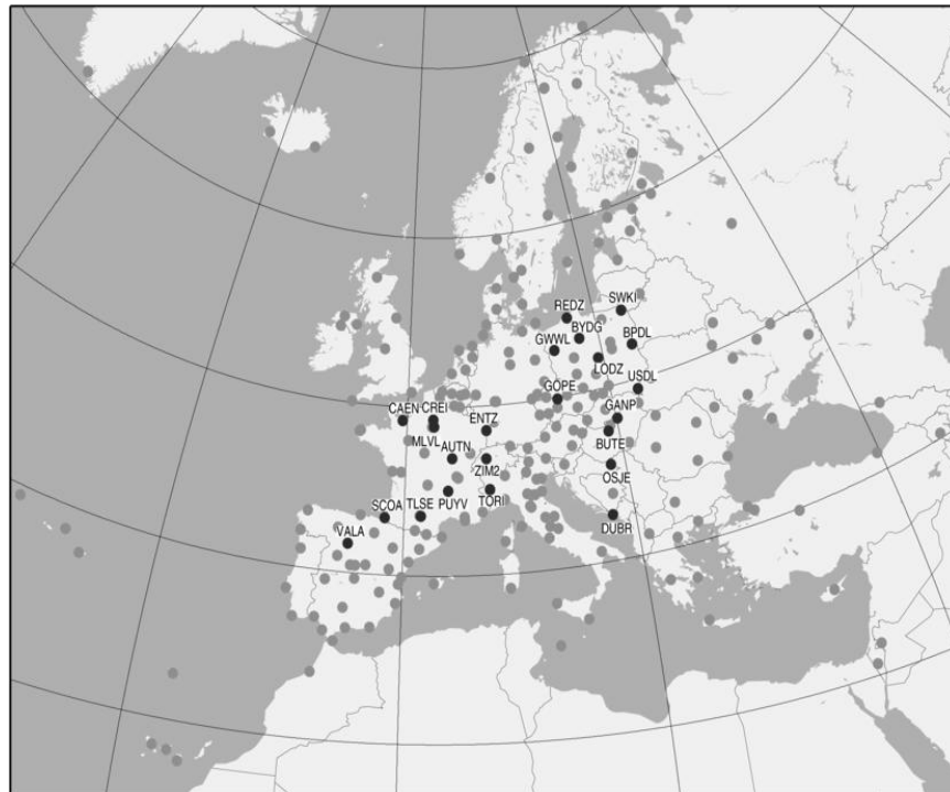
Figure 4 - EPN tracking network; stations indicated in dark (with label) track C2 (status June 1, 2010).
