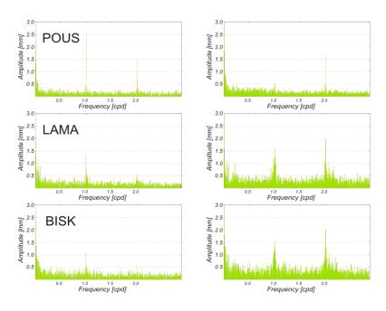
**Fig. 6** Periodograms of sites with oscillations in horizontal components (amplitude more than 1 mm), left: N-S component, right: E-W component.
