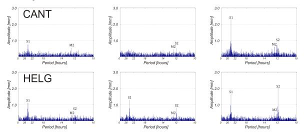
Fig. 10 Periodograms of coastal sites with oscillation in M2 frequency (from left: N-S component, E-W component, height ).
