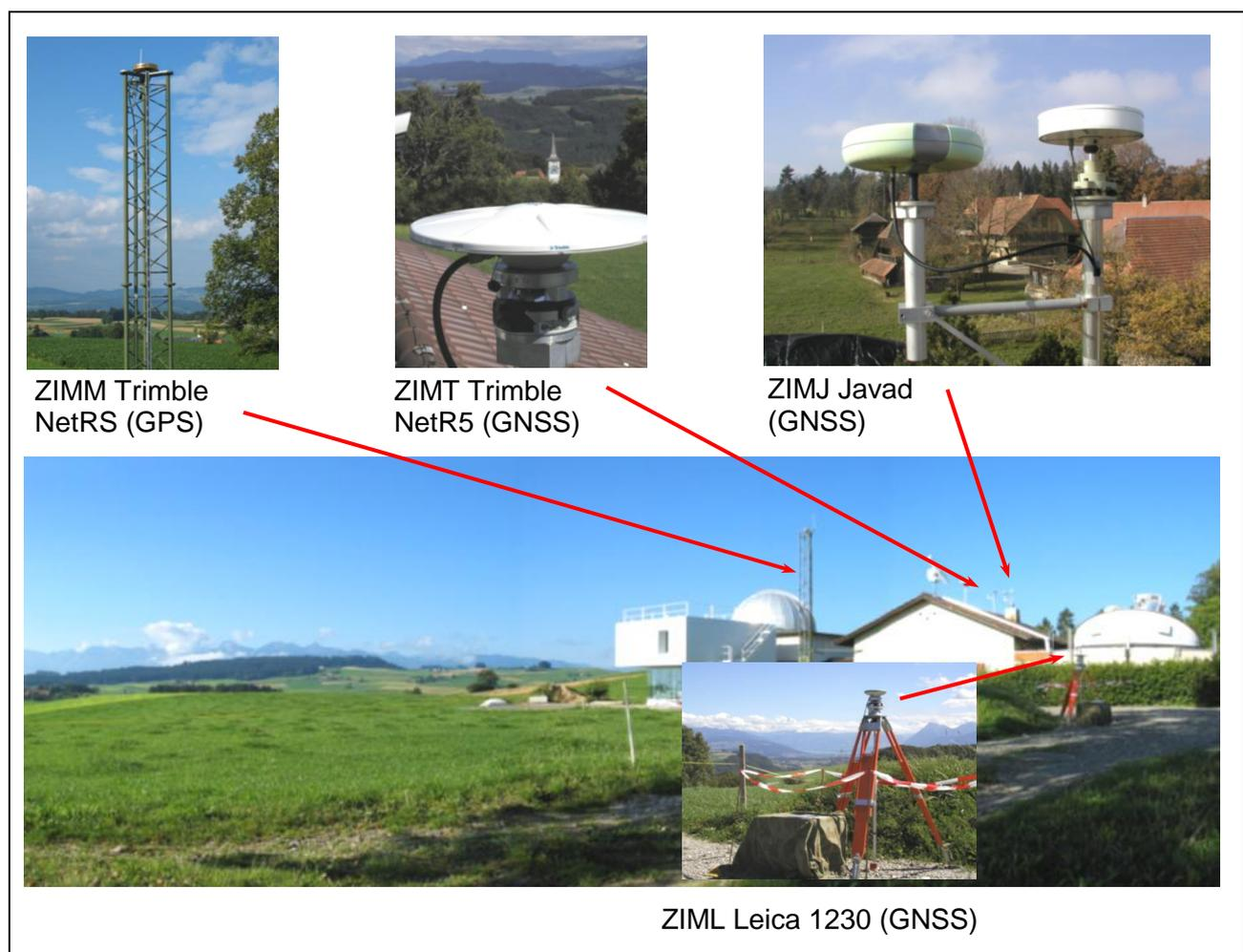
Figure 2: Antenna and receiver setup at the IGS site Zimmerwald (Switzerland) for the GNSS post-processing tests of short baselines with the Bernese GPS Software.
