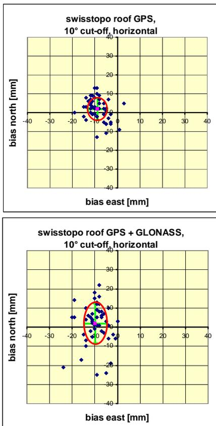
Figure 4: Coordinates and standard deviations (North and East) of RTK tests performed with a 10 degrees cut-off elevation angle. GPS-only results (top) and combined GPS/GLONASS results (bottom).
