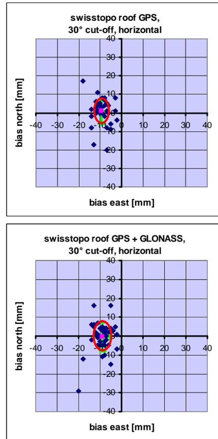
Figure 5: Coordinates and standard deviations (North and East) of RTK tests performed with a 30 degrees cut-off elevation angle. GPS-only results (top) and combined GPS/GLONASS results (bottom).
