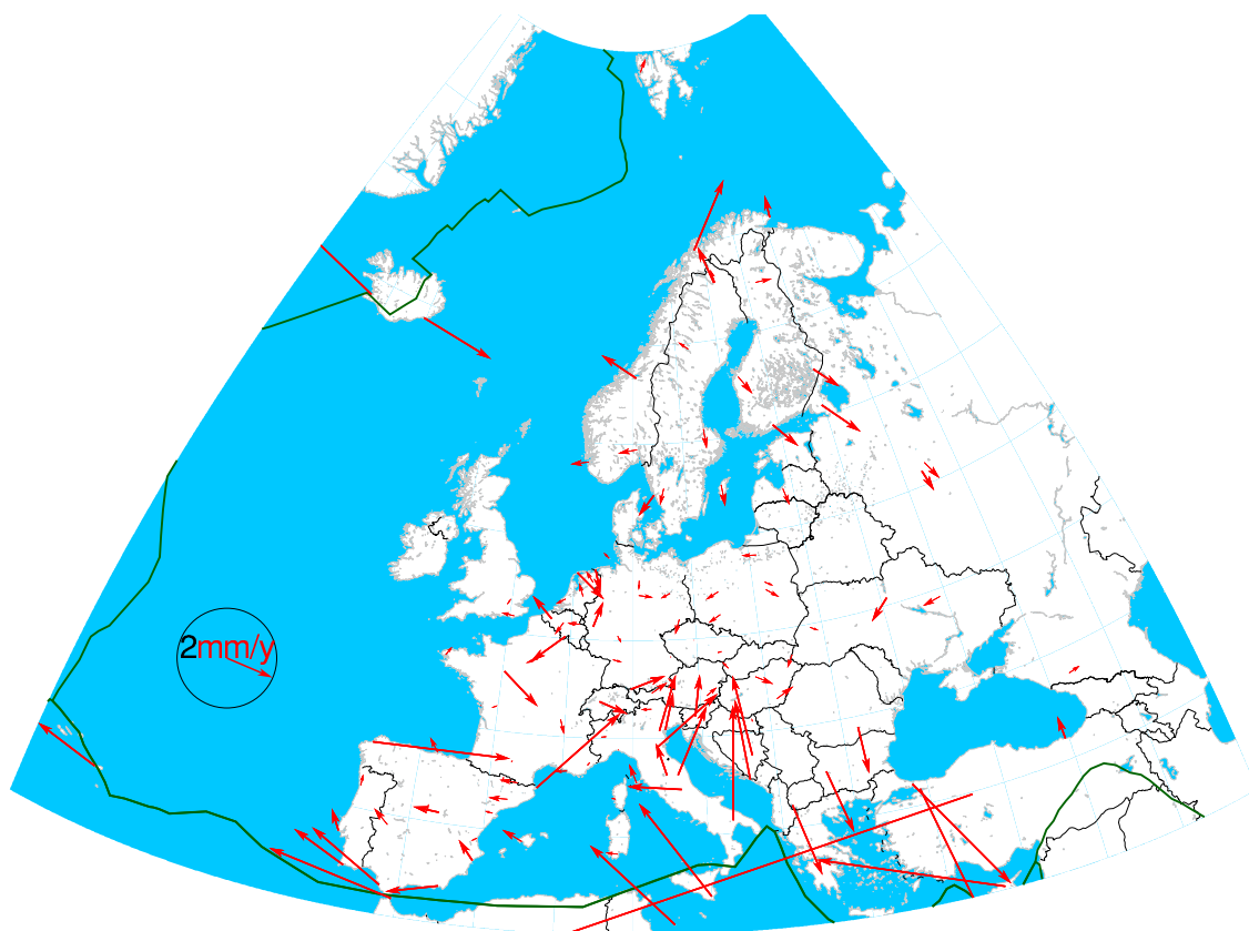
Figure 2. ETRF2000 horizontal velocities of EPN stations.
